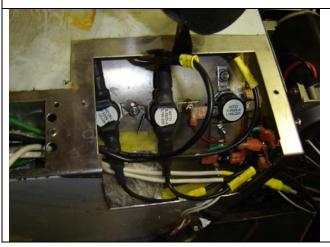
Screw in the new AC high limit aquastats. Use a little heat transfer paste under the aquastat if needed.
