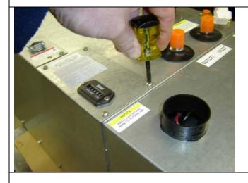
Unscrew the hour meter cover plate.
