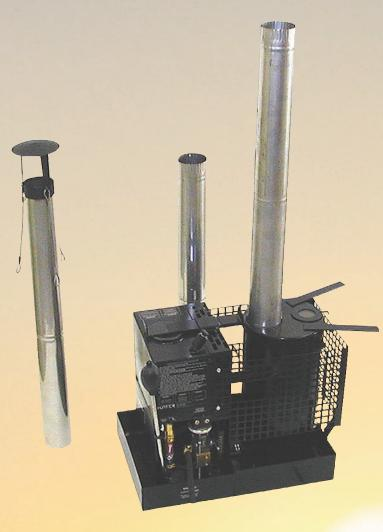
The Mini-Heater, SHS is individually packed, self contained, and produces 12,000 BTU from a compact, 11.5"W X 14"H X 17.5"D, lightweight, 32 lbs., unit. It incudes the fail-safe, non-flooding vaporizing burner which is controlled by adjusting the height of its carburetor. Designed for use with DF1, DF2, DFA, JP8, JetA1, and Kerosene.
