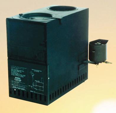
The Space Heater Arctic (SHA), is individually packed, self contained, and produces 23,000 BTU from a 9"W X 17"H X 17.5"D, 41 lb. unit. It incudes the fail-safe, non-flooding vaporizing burner which is controlled by adjusting an attached tri-viscosity fuel control valve. It is designed for use with DF1, DF2, DFA, JP8, JetA1, and Kerosene.
