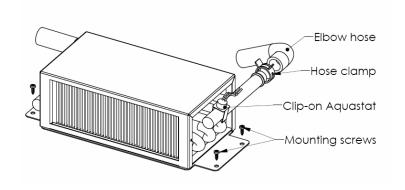
Figure 5-2: Mounting a Spacesaver Fan
