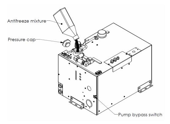
Figure 7-6: Initial fill up Oasis® Combi Heating System
