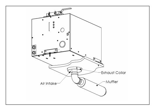
Figure 3-1: Installing the Exhaust System
