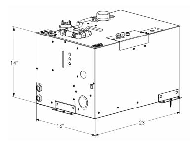
Figure 2-1: Oasis® Combi Heating System Dimensions
