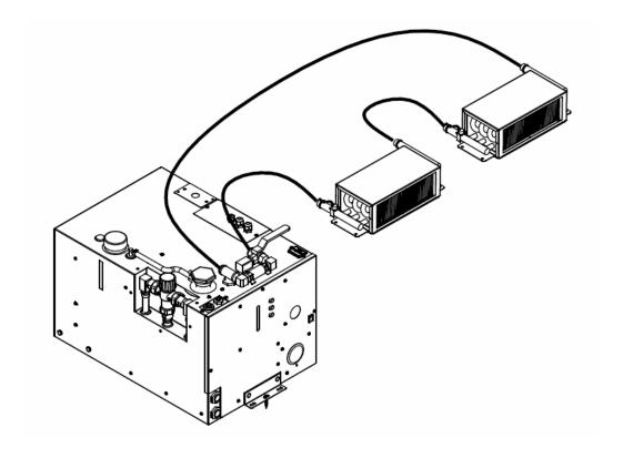
Figure 7-1 Oasis® Combi Heating System and cabin fans
