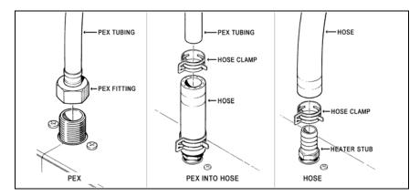
Figure 7-2: Three Approved Methods of Installing Heater Hose
