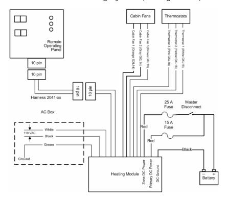
Figure 6-1 System wiring
