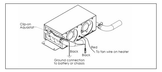
Figure 5-1: Wiring the Fan's Aquastat
