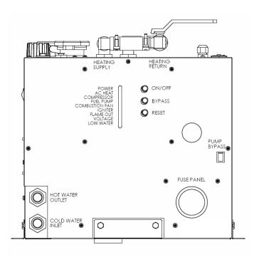
Figure 8-2 Combi Heating System Main Control Panel
