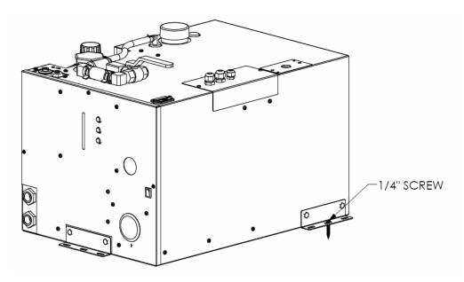
Figure 2-2: Oasis® Combi Mounting Brackets
