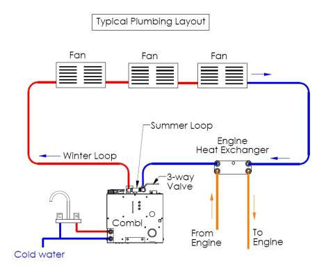
Figure 7-5 Engine Heat Exchanger/System Plumbing
