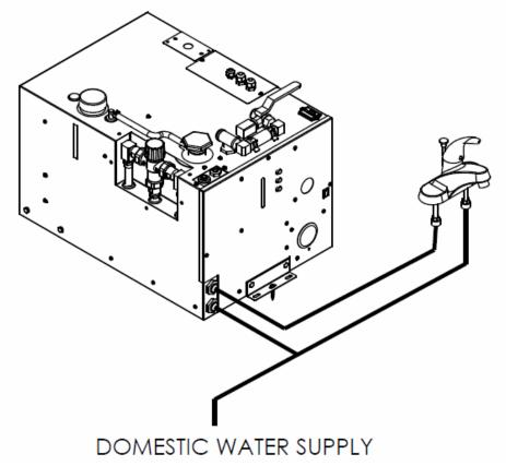
Figure 7-4 Domestic Hot Water System Plumbing.
