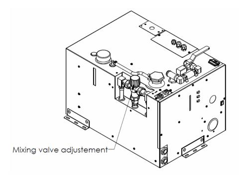
Figure 7-7: Mixing valve location
