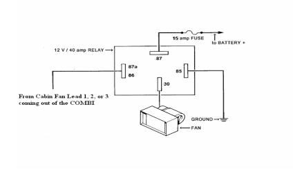
Figure 5-3: Installing a Relay for Additional Fan Amperage
